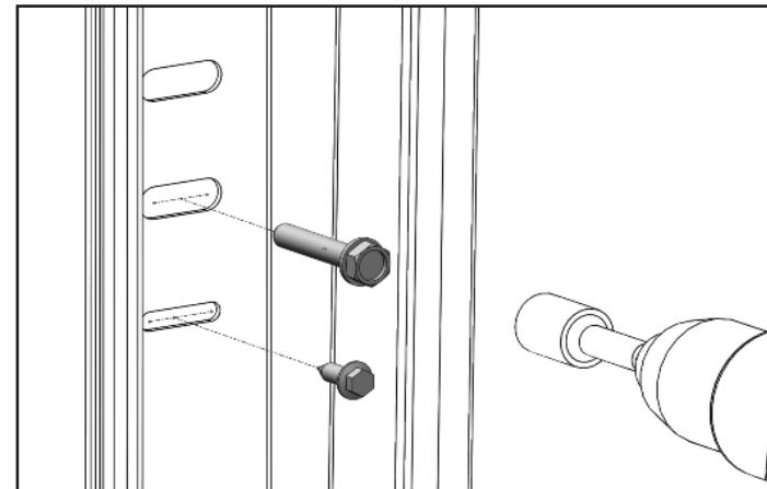
**E** Use brick or steel assembly set depending on frame material
