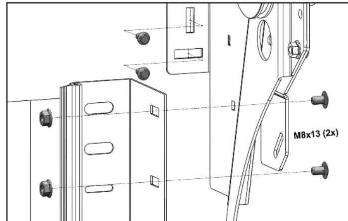
**E** Place the B20 08 bracket against the frame and against the outside of the vertical rail.
