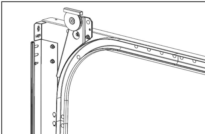
**E** Rail assembly with spring bar at the back
