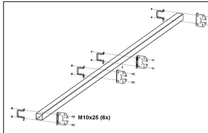
**E** Fit the horizontal rail with bend on the bracket and vertical rail
