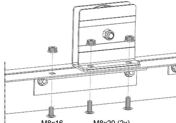
**E** Install the spacer profile to the guide bracket. Doors larger than 5000 mm only.
