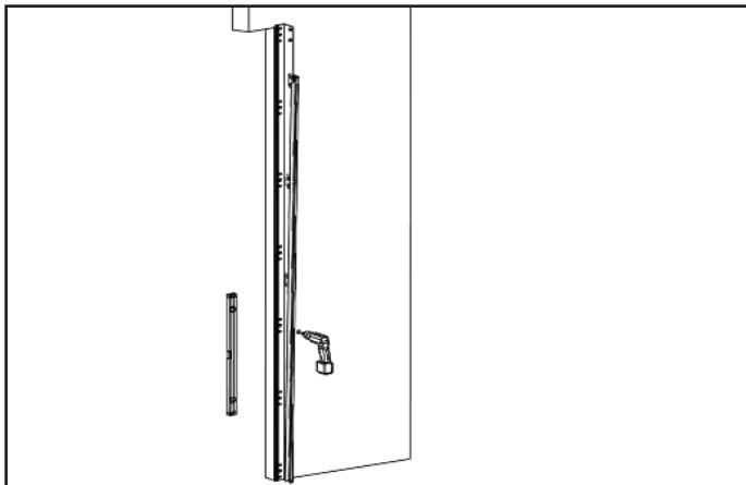
**E** Place the vertical rail level against the frame at the correct width
