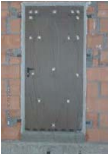
A test object mounted to a test wall and the positioning of the sensors.
